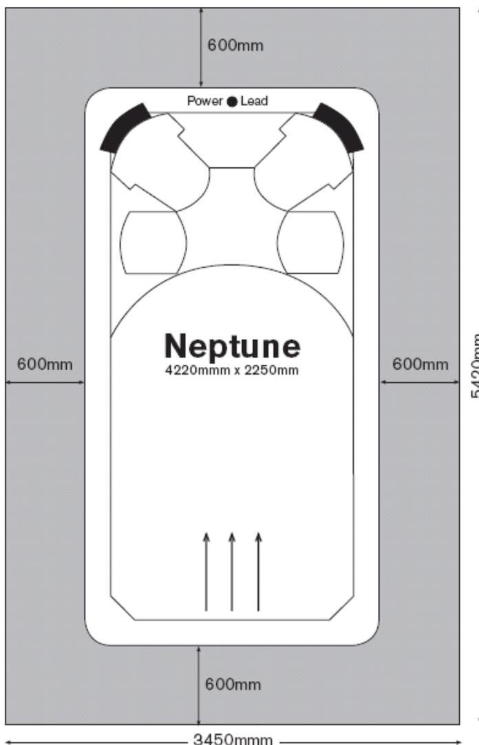
**In Decking:** If you are sinking your pool and decking around it please remember to build the decking to allow access to the electrical compartment and all components. Please ensure the electrical compartment has some ventilation for correct functioning. If decking up to/around pool, we would recommend decking after installation.
