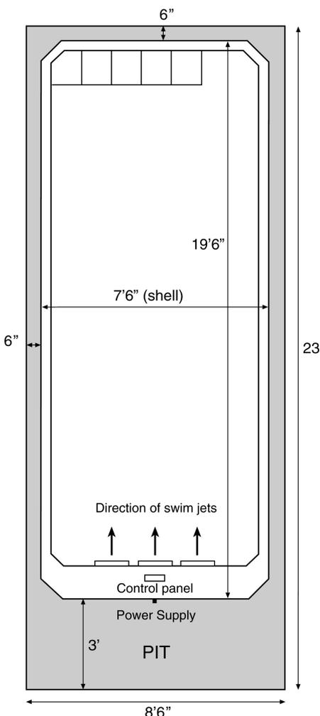
**In Decking:** If you are sinking your pool and decking around it please remember to provide a trapdoor in the decking to allow access to the electrical compartment. Please ensure the electrical compartment has some ventilation for correct functioning. If decking up to/around pool, we would recommend decking after installation.
