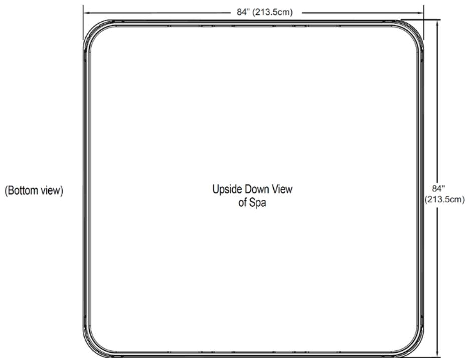
**NOTE:** Watkins Manufacturing Corporation recommends that the **FLAIR** be installed on a minimum 10 cm thick reinforced concrete pad or structurally sound deck able to support the "dead weight" found in the spa specification chart.
