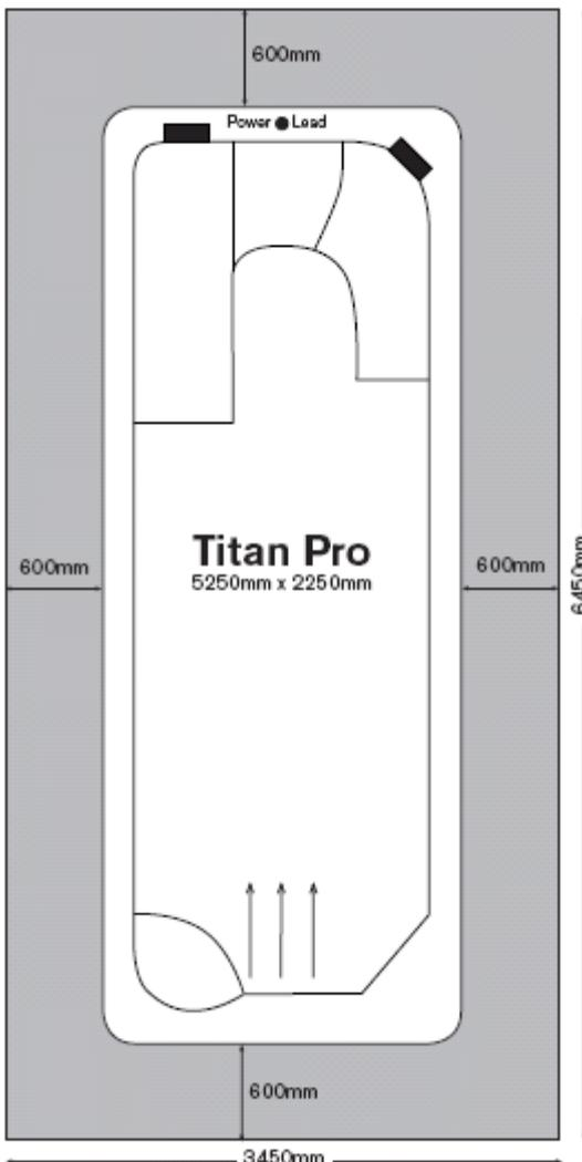
**In Decking:** If you are sinking your pool and decking around it please remember to build the decking to allow access to the electrical compartment and all components. Please ensure the electrical compartment has some ventilation for correct functioning. If decking up to/around pool, we would recommend decking after installation.
